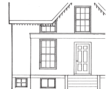
Inappropriately enclosed porch.
