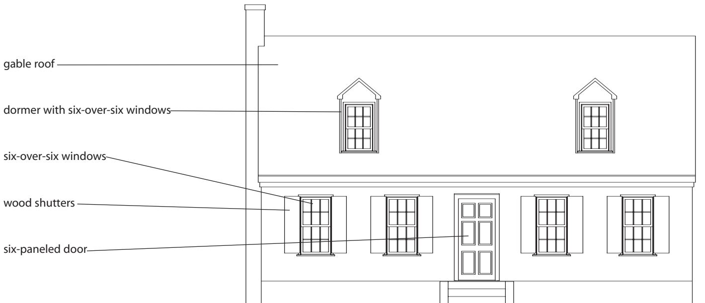
One-and-a-half-story Colonial Revival
