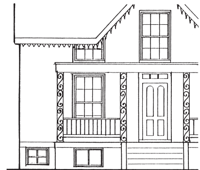
Inappropriately remodeled porch.
