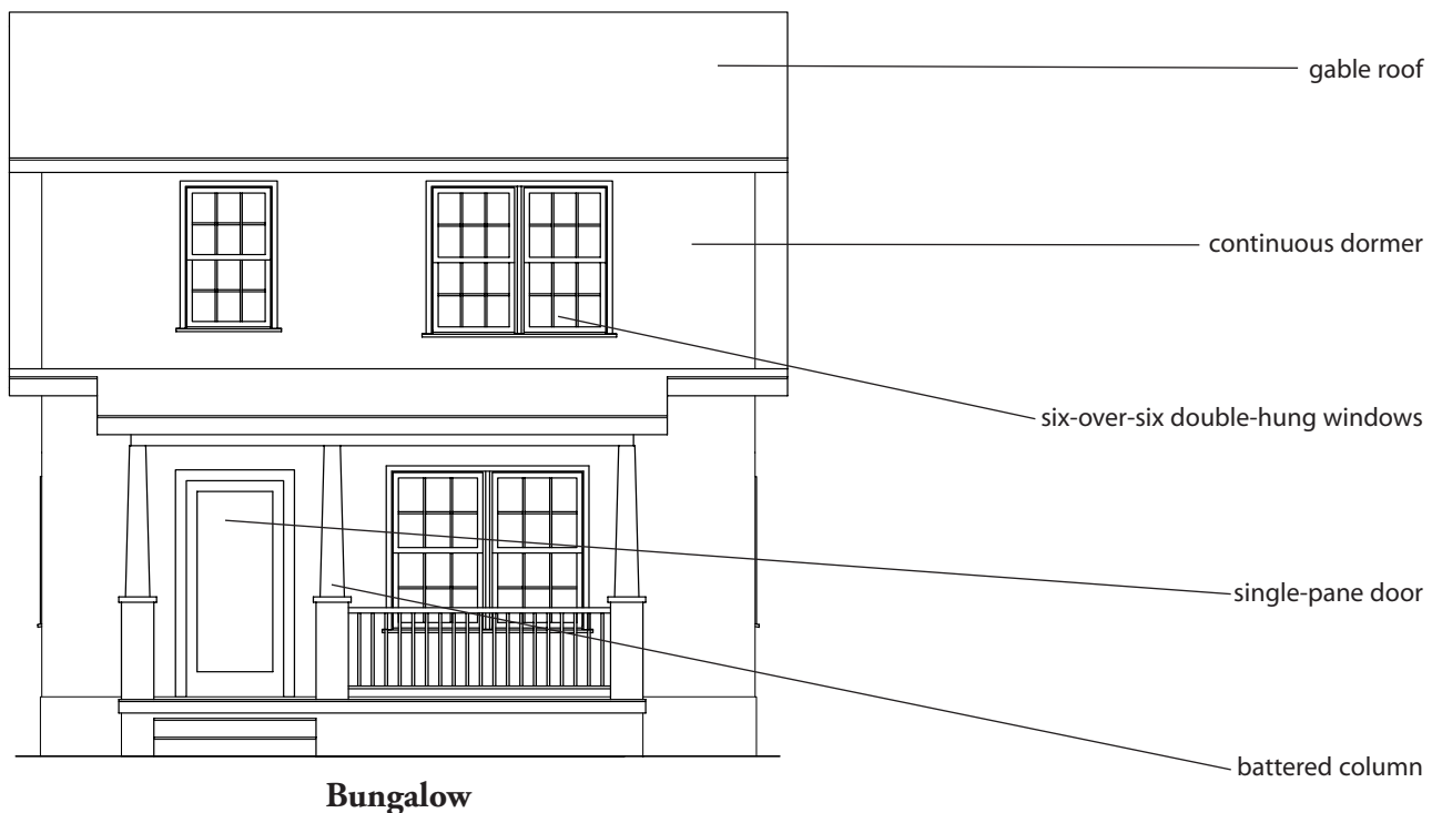
A continuous shed dormer spans the width of this bungalow and echoes the grouped six-over-six windows on the first floor. Short wood columns rest on brick piers to support the full width front porch.
