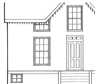
Inappropriately removed porch.
