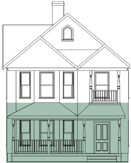
New residences in the historic district should have porches based on historical precedent.
